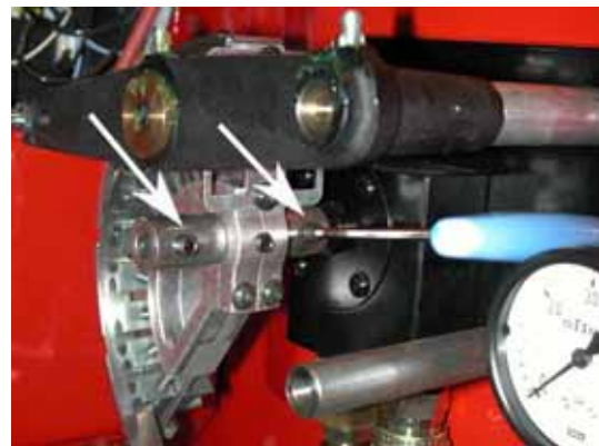
6. Loosen the locking screws on the oil regulator shaft.
