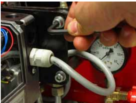
5. Unscrew the screws holding the servomotor mounting plate. Pull out the servomotor. Place and fasten the servomotor so that there is no stretching strain on the cables.
