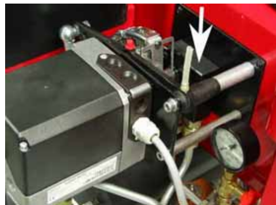
2. The oil regulator valve is located between servomotor and the burner body. See arrow.
