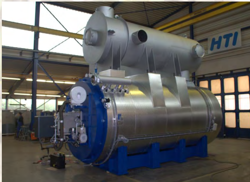
Natural Gas Fired Heater w. Economizer – 4.000 kW
