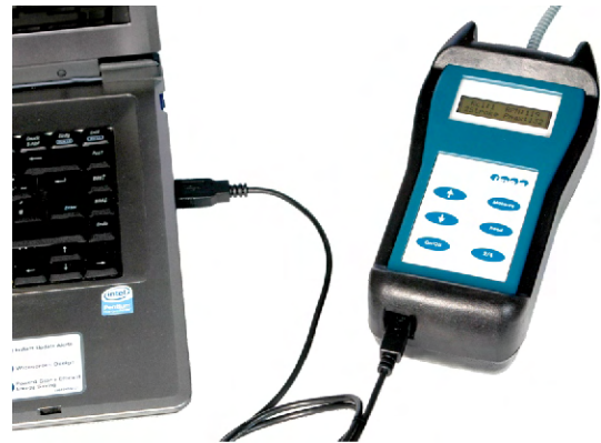
EPM-XP connected via USB cable to notebook for quick data download and for charging 9 V block battery
